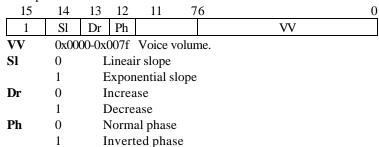
In sweep mode, the current volume increases to its maximum value, or decreases to its mimimum value, according to mode. Choose phase equal to the the phase of the current volume.
