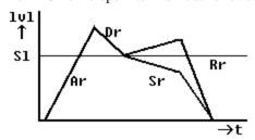
**Ar** Attack rate, which specifies the speed at which the volume increases from zero to it's maximum value, as soon as the note on is given. The slope can be set to lineair or exponential.
