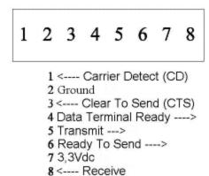
The pot speed is able to go up to a maximum of 256K bps. Normally it's used at 56K. On connecton problems the port will attempt a reconnect, but may not fall back on a slower speed. The link cable is wired is such.
